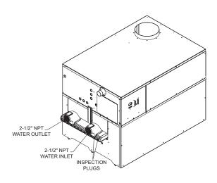
FIG. 32 Water Connections
